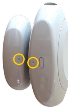
Figure 82: Dot Alignment of the Magnetic Sensor Units
