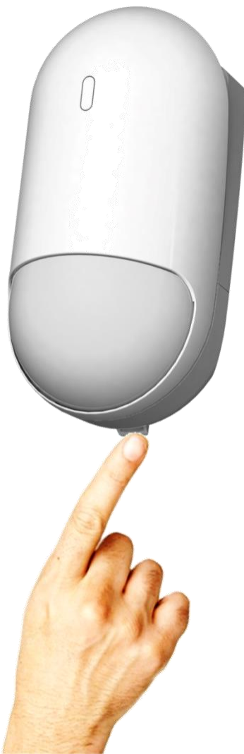
Figure 72: Dismounting the Motion Detector
