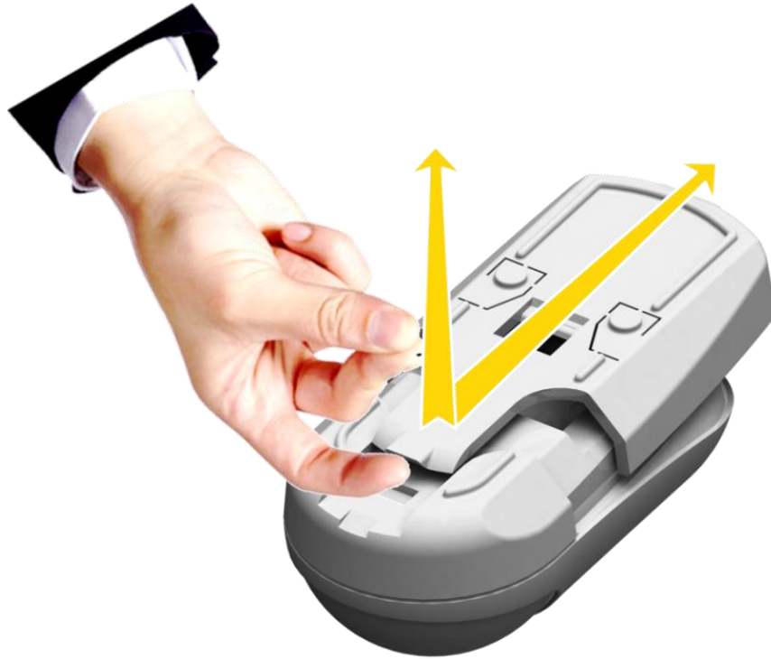
Figure 70: Releasing the Motion Detector Wall Mounting Base
