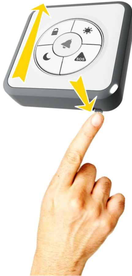
Figure 207: Dismounting the Tag Reader
