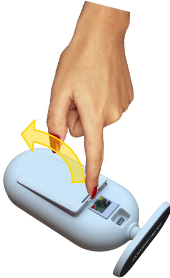
Figure 192: Releasing the Back Cover
