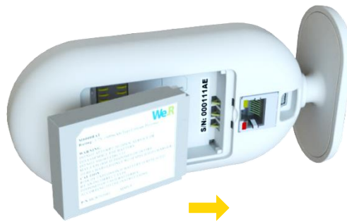
Figure 194: Insertion of the Backup Battery
