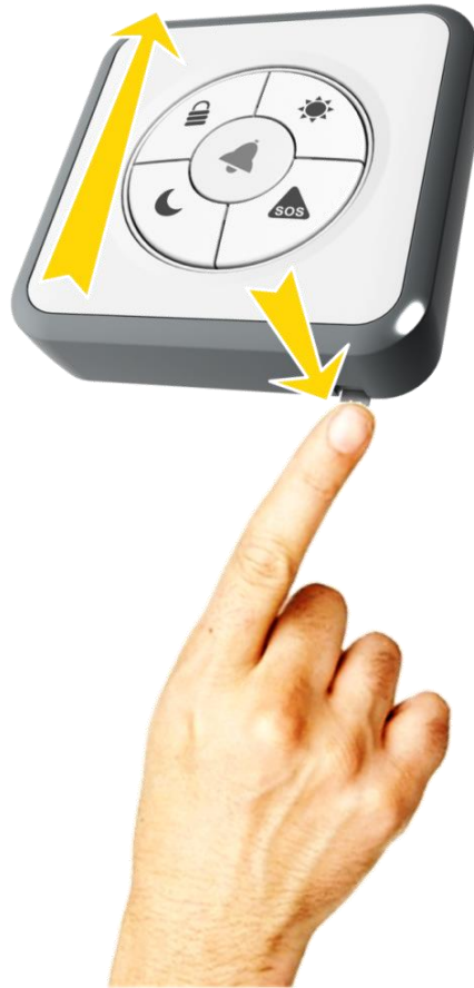
Figure 103: Dismounting the Tag Reader
