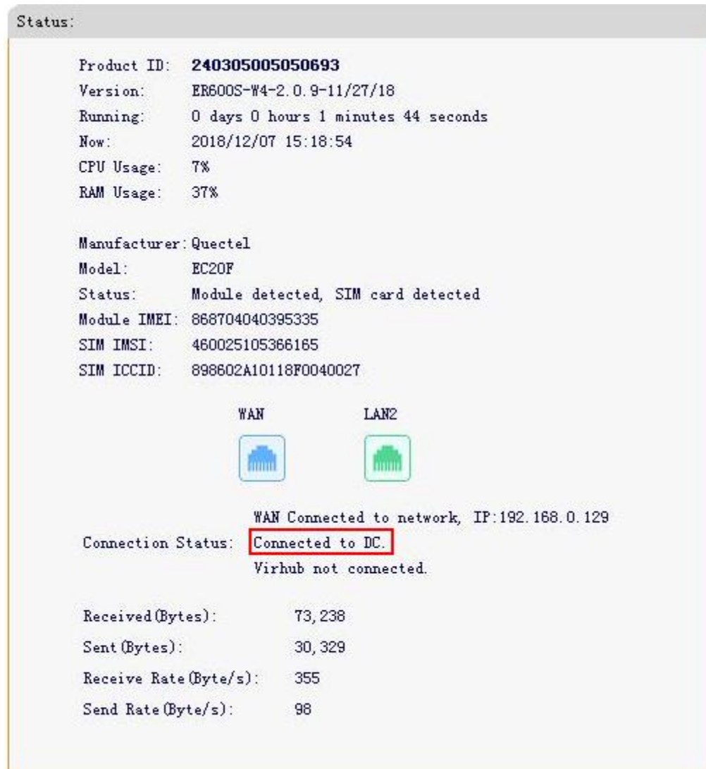
Figure Appendix 4-4: DTU connected to DC
