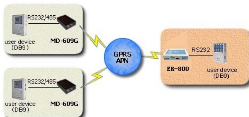
Figure Appendix 3-1: Embedded data center and APN network solution
