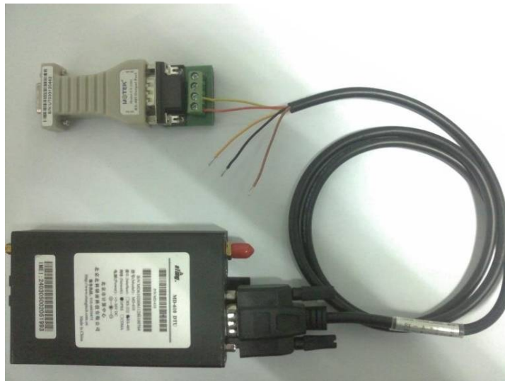
Figure Appendix 3-6: 9-pin adapter connection diagram
