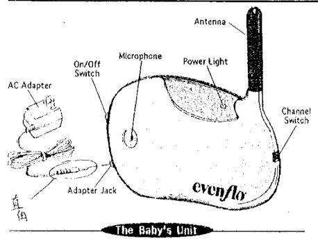
The Baby's Unit is a transmitter, which sends sounds to the Parent's Unit (receiver). It is powered either a 9 volt battery or by an AC adapter which is included.
