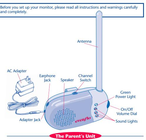
The Parent's Unit receives sound from the Baby's Unit (transmitter) and is powered either by three AAA batteries or by an AC adapter which is included.
