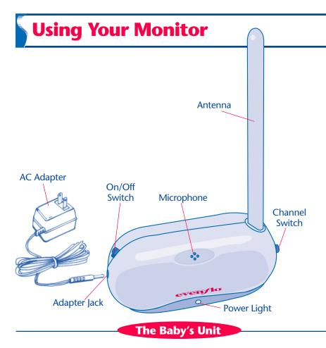
The Baby's Unit is a transmitter, which sends sounds to the Parent's Unit (receiver). It is powered either by a 9 volt battery or by an AC adapter which is included.
