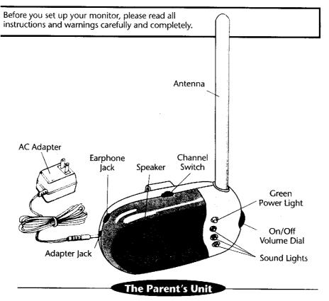
The Parent's Unit receives sound from the Baby's Unit (transmitter) and is powered either by three AAA batteries or by an AC adapter which is included.
