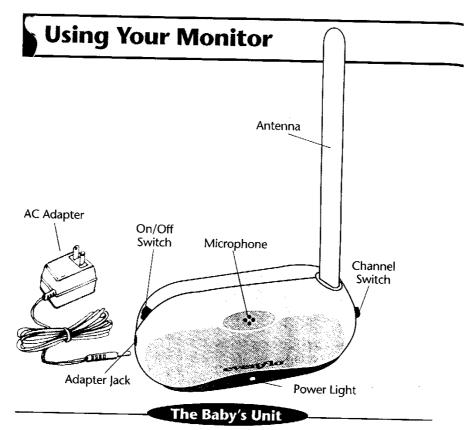
The Baby's Unit is a transmitter, which sends sounds to the Parent's Unit (receiver). It is powered either by a 9 volt battery or by an AC adapter which is included.
