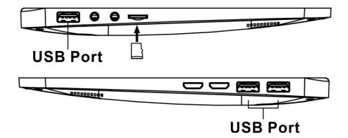
This device supports USB devices such as USB thumb Drive to increase the memory size and to read files, simply insert the device into the USB port as indicated in above.
