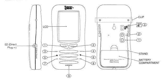
S2 (Direct Plug in) - allows you to plug 1 detachable stainless steel probe sensor directly into the receiver unit.
