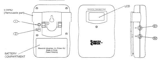
STAND - Swings out and allows you to stand receiver on tabletop.
