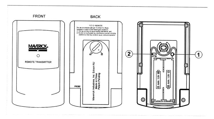
BATTERY COMPARTMENT - holds 2 AAA batteries.
