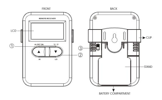
LCD (Liquid Crystal Display) – Displays all icons, temperature. See LCD diagram for detailed information.
