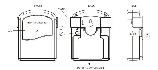
STAND - Swings out and allows you to stand receiver on tabletop.
