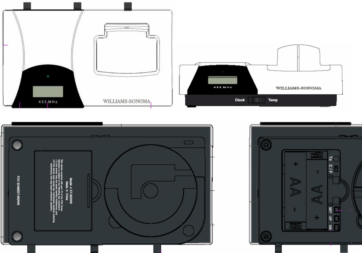
BATTERY COMPARTMENT – holds 2 AA batteries.
