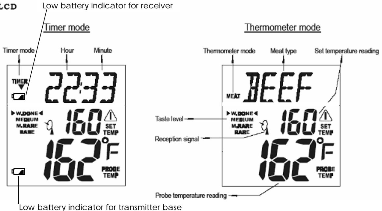
In thermometer mode, the main unit displays the food temperature measured by the remote sensor and prompts the user about the cooking level.
