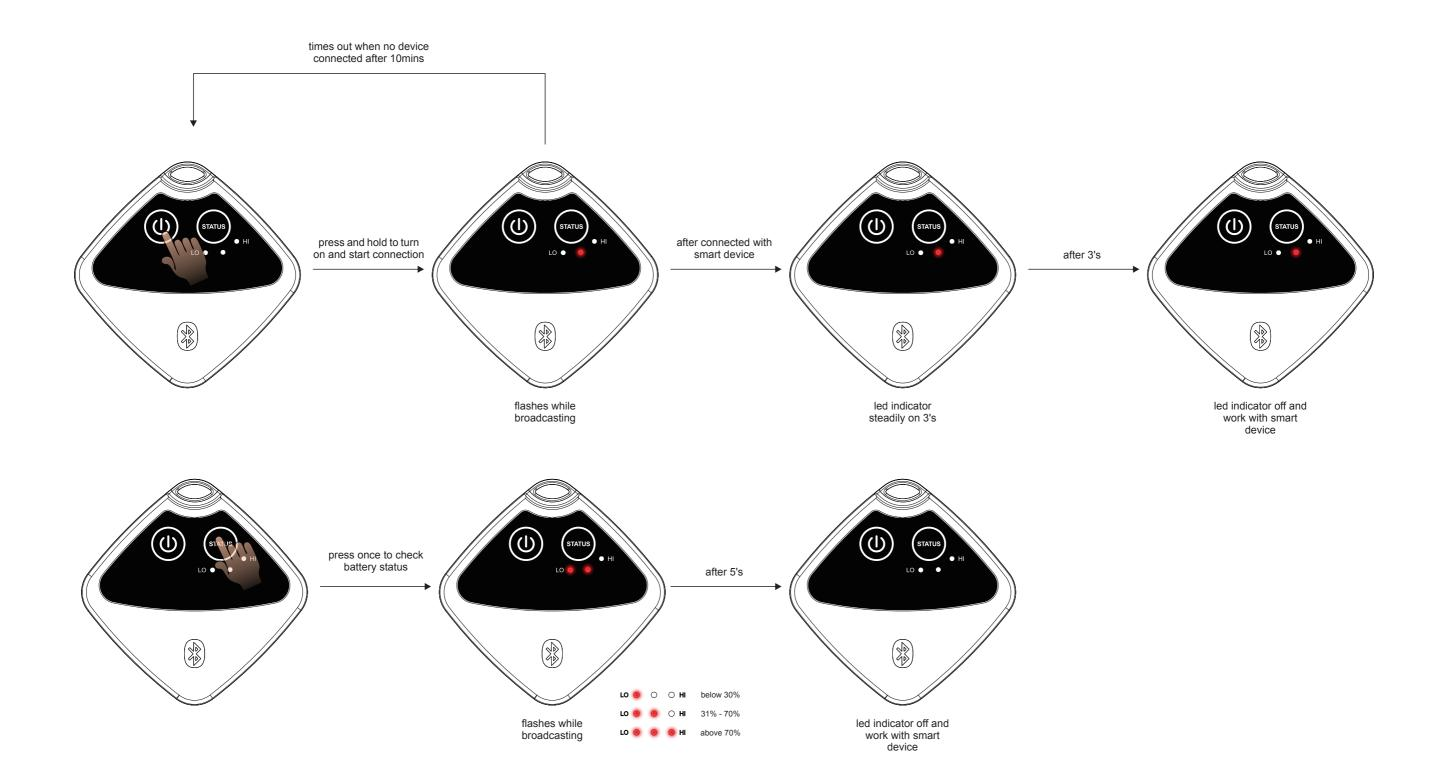
Specifications 1.Voltage Supply: 1 x CR2032 3.0V Lithium battery 2.Temperature Range: -20 to +60 °C 3.Recording cycle: up to 22 days (with 1min sampling time interval) up to 45 hours (with 5sec sampling time interval) 4.Battery life: 12 months \* depends on data sampling rate setting 5.Protection class: IPX4 6.Indicator: 1 x LED (red) to show pairing and battery stauts 7.Dimensions: (W)49 x (H)49 x (D)11.5mm 8.Weight: Approx. 15g
