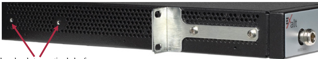
Figure 4-3: Rear-mount hole locations
