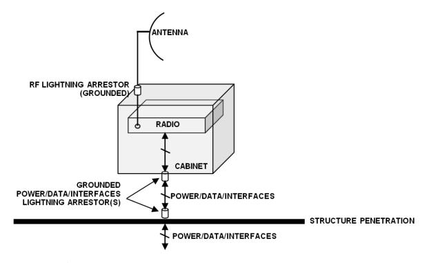
Figure 3 Enclosure mount interconnection
