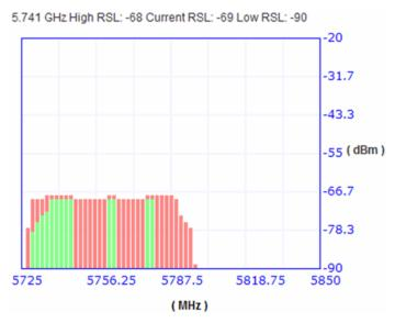
Figure 52 Spectrum analyzer graph example
