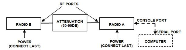
Figure 65 Basic back-to-back bench test configuration
