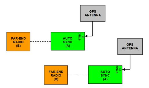
Figure 8 Synchronized GPS sources using AUTO SYNC
