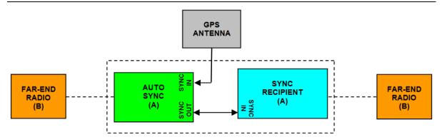
Figure 7 GPS as primary sync source using AUTO SYNC
