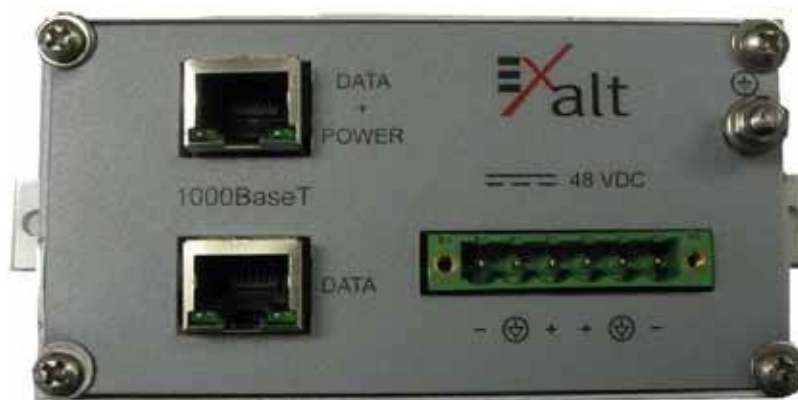
Figure 14 Power injector connectors
