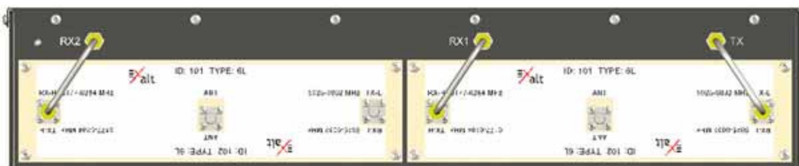
Figure 14 Typical Space Diversity diplexer configuration
