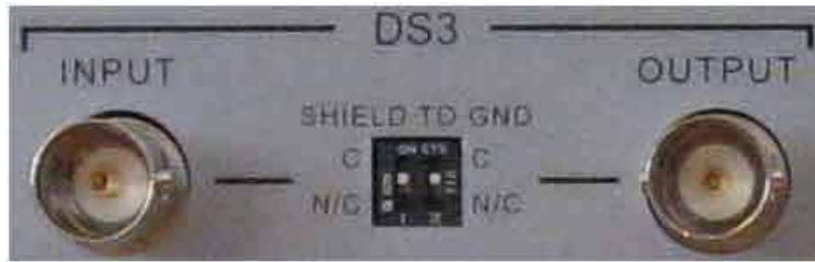
Figure 10 DS3 connectors and grounding switches
