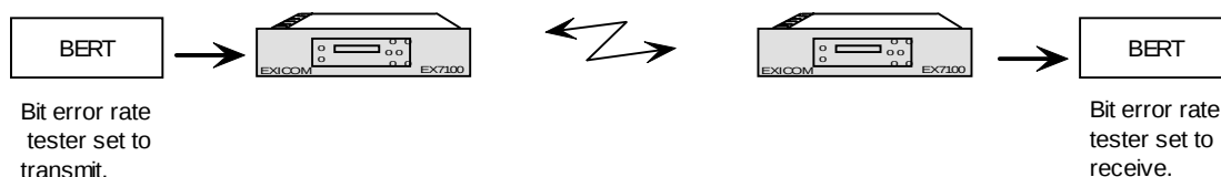
Figure 4.5: End-to-End Bit Error Rate Test
