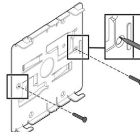
**Note:** The 4 feet of the bracket must be horizontal and pointing to the right and the flat part of the bracket must be touching the surface it is being attached to.
