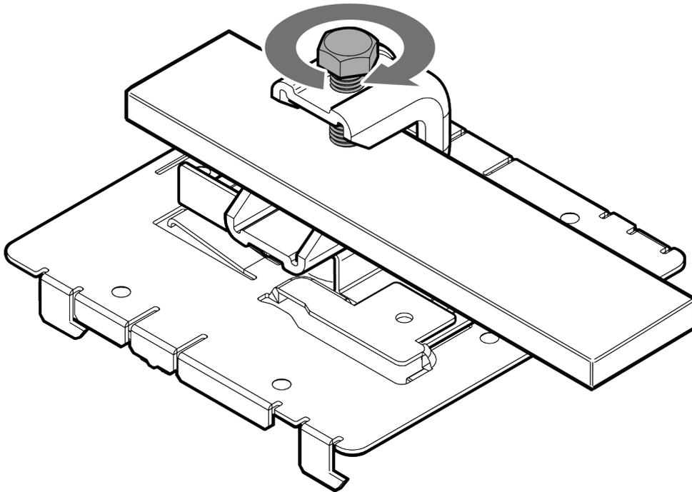
**Figure 10: Beam clip accessory attached to a beam**
