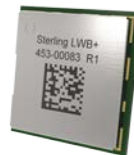
Wi-Fi 5 and Bluetooth v5.2 embeddable SiP
