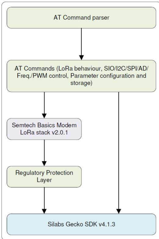
Figure 7: Firmware block diagram - AT firmware
