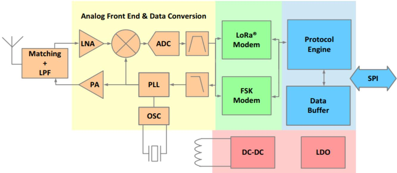
Figure 3: SX126X Block Diagram (from SX1261/SX1262 Datasheet)
