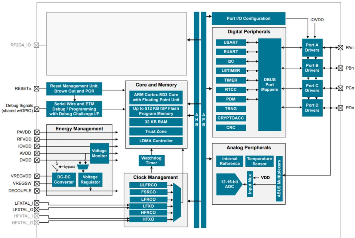
Figure 4: EFR32BG22 microcontroller peripherals and block diagram (from EFR32 datasheet)
