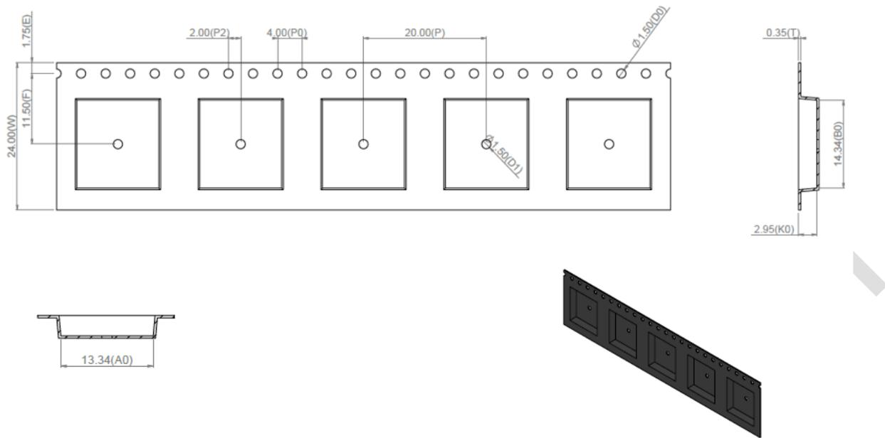
Figure 14: RM126x Carrier Tape Specifications
