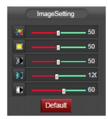
You can set the color parameters for the video image in this "ImageSet", such as Hue, Brightness, Contrast, Saturation, Sharpness.
