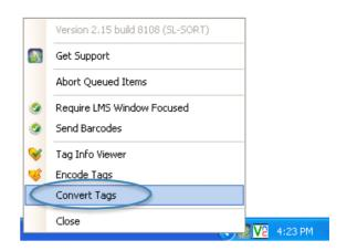
When items of the old tag data format are detected, a window will be displayed onscreen prompting you to provide any necessary tag parameter information for the new tag data format. After the tag parameters have been provided, clicking the "OK" button will proceed to convert the tag to the new tag data format.
