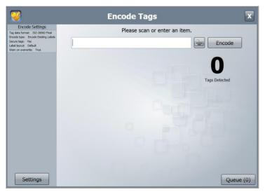
This function can be used to encode RFID tags. Tags can be placed on the RFID pad and encoded with the required data.
