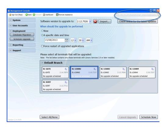
By pressing this button, Management Console will inform the user if a newer version of the software is available and prompt them to download it. Upon the download completing, the version number corresponding to the installation package will be visible within the *Software version* list box control.
