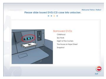
• If DVD cases that have not been borrowed are inserted in the unlocker, a message will appear on the computer screen, the unlocker will emit a red light and an audible alarm and the patron will be unable to fully insert the DVD case into the unlocker to unlock it.
