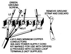
1. Remove the access plate near the cord set entry hole.
