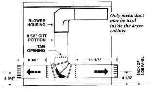
NOTE: To secure the duct, insert the tab (located on the appliance base) in the opening and bend it.
