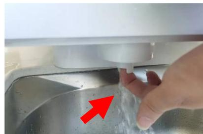
3. Use a pump to empty the disinfectant tank.
