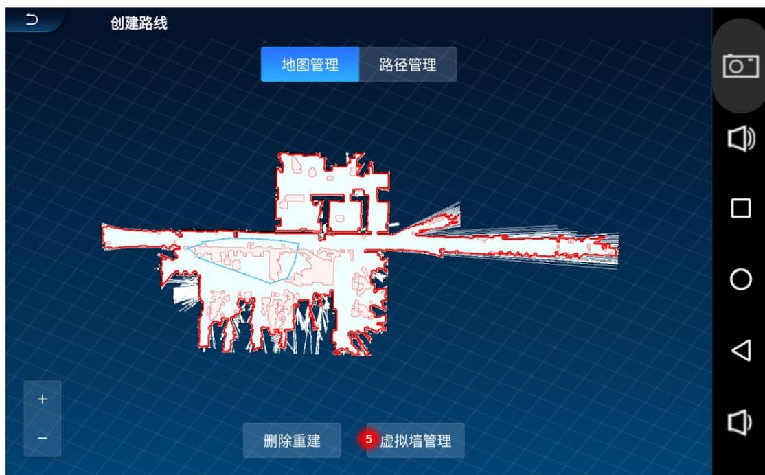
(6) Click to confirm the starting point and ending point of the virtual wall. Click “+” to draw a new virtual wall. Click “↶” to undo, and click “🗑️” to delete.
