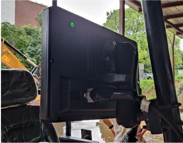
Connect the main harness, the body sensor, and the power harness to the corresponding ports. Then, turn on the switch on the power harness to check whether the power indicator of the control terminal is lit, and turn on the control terminal to check whether it works normally.
