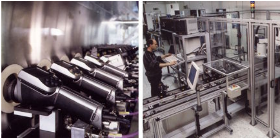
Figure 29.5 LEFT: Testing of infrared cameras in the climatic chamber; RIGHT: Robot used for camera testing and calibration
