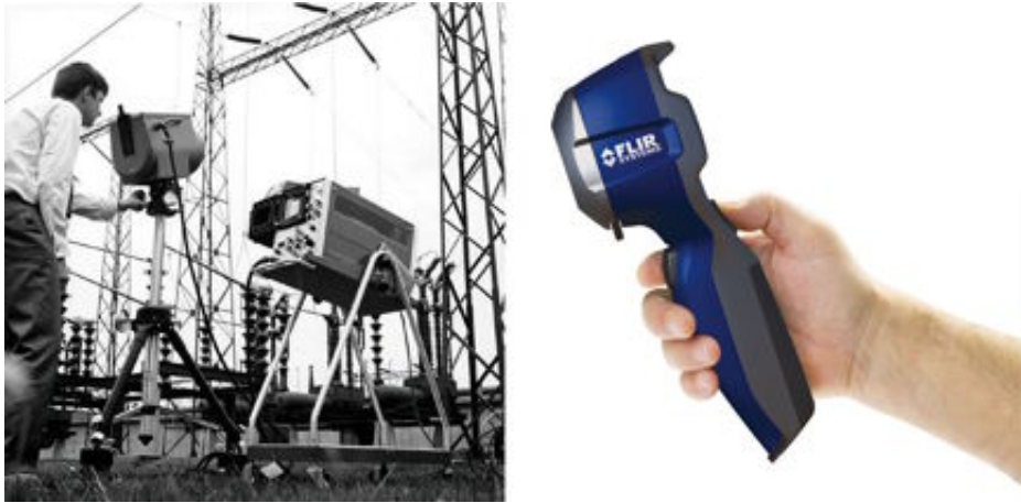
Figure 29.2 LEFT: Thermovision® Model 661 from 1969. The camera weighed approximately 25 kg (55 lb.), the oscilloscope 20 kg (44 lb.), and the tripod 15 kg (33 lb.). The operator also needed a 220 VAC generator set, and a 10 L (2.6 US gallon) jar with liquid nitrogen. To the left of the oscilloscope the Polaroid attachment (6 kg/13 lb.) can be seen. RIGHT: FLIR i7 from 2009. Weight: 0.34 kg (0.75 lb.), including the battery.
