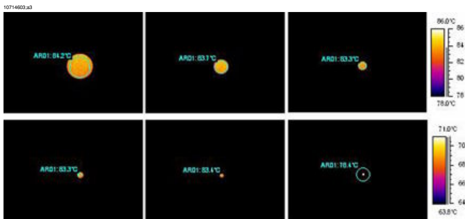
Figure 28.20 Temperature readings from a blackbody at +85°C (+185°F) at increasing distances (24° lens)
