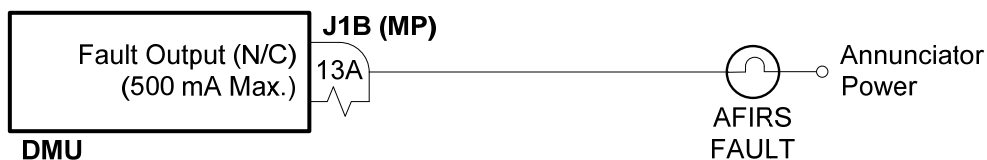
Figure 7-3 – Fault (N/C) Interface
