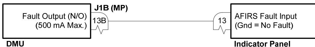
Figure 7-4 – Fault (N/O) Interface
