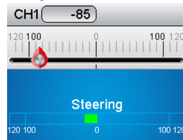
Subtrim setting and channel's current position
