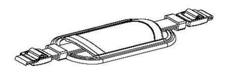
The Hand Strap may be attached between any of the four anchor points at each corner of the tablet. Thread each end of the strap into the anchor from the back side of the tablet, fold over, tighten and secure in the strap buckle. Tuck extra lengths into the grip sleeve.
