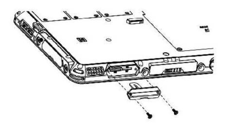
Remove screws securing the rubber seal protecting access to the 3G SIM and Micro SD card. Orient either card so the gold contact edge faces toward the front of the tablet and slide in the appropriate slot until it clicks in place.
