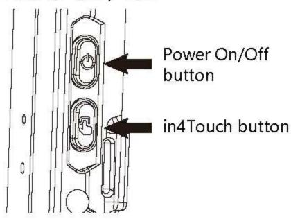
Press and hold the Power On/Off button for 2 seconds to turn on the system. You will feel a vibration. Press and hold again for 5 seconds to turn off the system, but only if unable to turn off normally through software.
