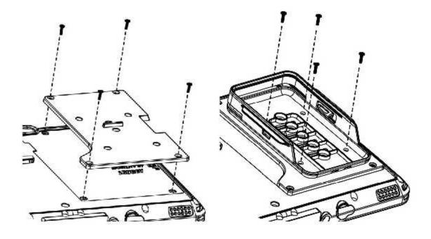
Position the universal mounting plate over the battery module as shown and attach with 4 screws provided. Then attach the mPOS bracket to the mounting plate with 4 additional screws.
