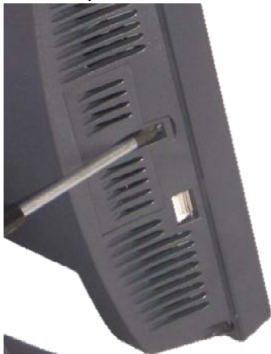
HDD access panel
