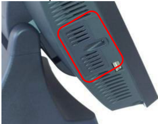
HDD access panel
