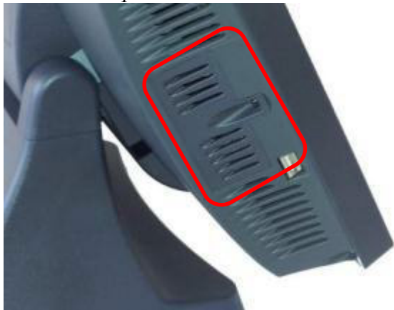
HDD access panel
