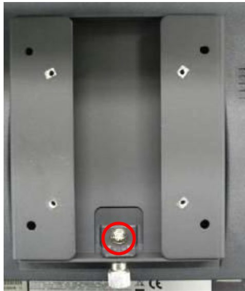
Install screw to secure thumbscrew clip
