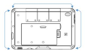
Use of the standard hand strap shipped with the tablet is optional. Depending on the situation, the user may attach the hand strap between anchor points across the top or either side of the tablet. To attach the strap to the tablet, thread both ends of the strap into an anchor point, fold back and tighten in the plastic buckle. Any excess can be tucked into the sleeve handle at the center of the strap.
