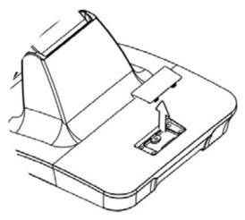
To install the customer display, remove the single screw securing a cover over the rear mount area and discard.
