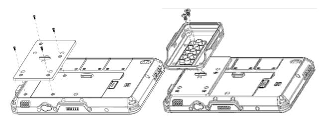
To attach the bracket, place the tablet face down. Position the metal universal mounting plate over the battery module as shown and attach with the four screws provided (you may need to first remove and discard cosmetic rubber covers placed over the screw holes).
