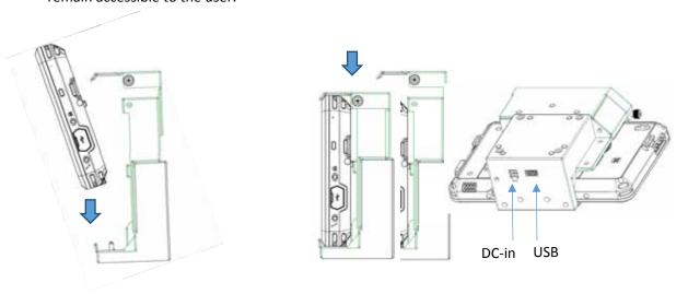
To place the tablet in the mount, first raise the top arm of the mount. Angle the unit from the bottom as shown. Slide the arm down and secure.
