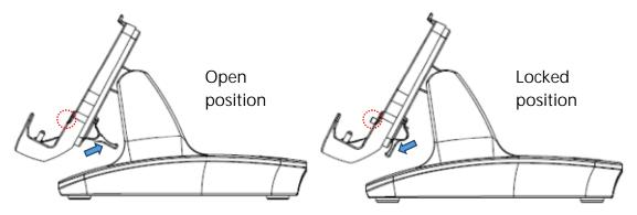
There is a latching mechanism to secure the tablet in the dock, accessed on the back of the mount. Before placing the tablet in the dock, check to make sure the latch is in the open position.
