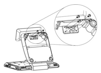
Thread the customer display cable through the opening and fasten the display mount into place with the four screws provided. Connect the host end of the cable to any of the available USB ports.
