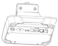
Disconnect the power cable from the docking station. Plug network or peripheral cables into available ports located in the base:
