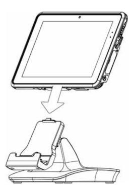
The tablet may be placed on the dock powered on or off. When positioning the tablet on the dock, take care to locate the extension on the back center of the tablet and make sure this slides over the tab on the mount.
