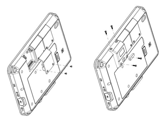
Remove the two screws and lift off the plastic cover covering each bay. This cover may be saved or discarded. Slide the module in place and fasten in place with the four screws provided.
