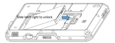
Next slide the latch holding the main battery module in place and lift out the battery at an angle as shown above.
