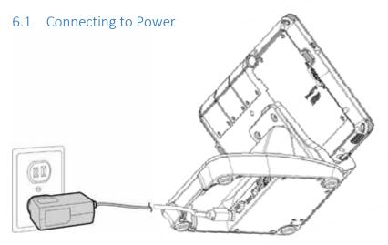
Before the docking station can be used to charge the tablet or connect to peripherals, the dock must be connected to AC power via the 19V/65W AC adaptor shipped with the POS Dock. Locate the DC-in connector on the dock and plug in the power cable from the AC adaptor.
