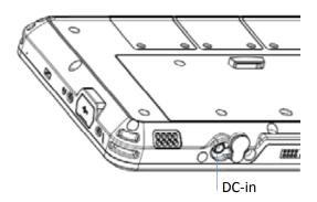
The battery may be charged by connecting the supplied AC power adaptor directly to the DC-in connector located on the bottom of the tablet. Push the protective rubber seal aside and plug the cable directly into the connector. Then plug the adaptor directly into the AC outlet.
