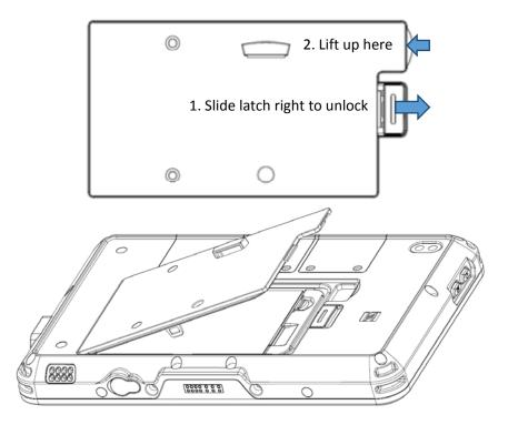
The main battery module may be removed by releasing the latch and lifting up the access cover as shown above.
