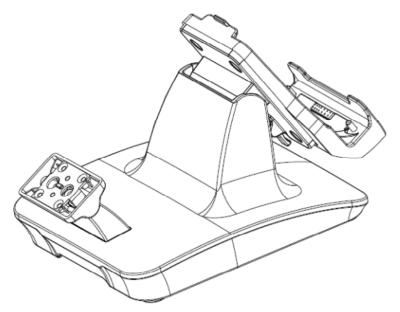
To install the device mount, remove the screw and discard the blanking cover over the rear mount access. Attach the post to the base with the four screws provided before attaching the iRuggy Systems mPOS bracket.
