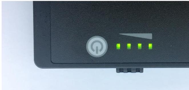
With the battery module removed from the unit, press the icon shown above. The row of LEDs will light up for 3-4 seconds indicating battery charge level as follows:
