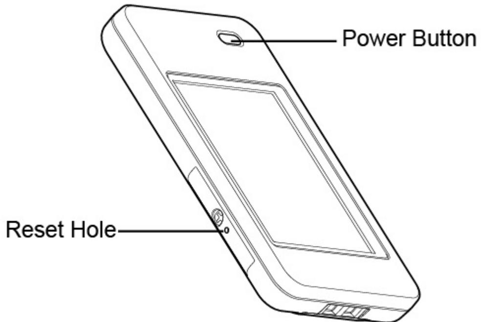
1. Use a tool to gently press the “Reset Hole” once on the side of the mobile system while keep holding down the “Power Button” throughout until the system lead you to the calibration instruction window.
