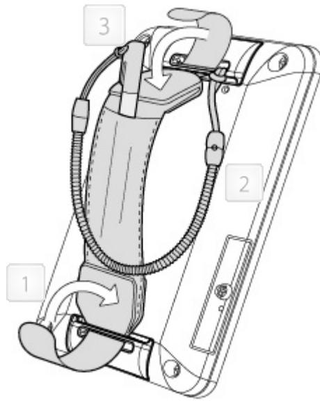
1. Thread the hand strip through the strip rings on the rear top and rear bottom sides of the system. Fix the hand strip by pressing the velcro at two ends. (as arrows shown)
