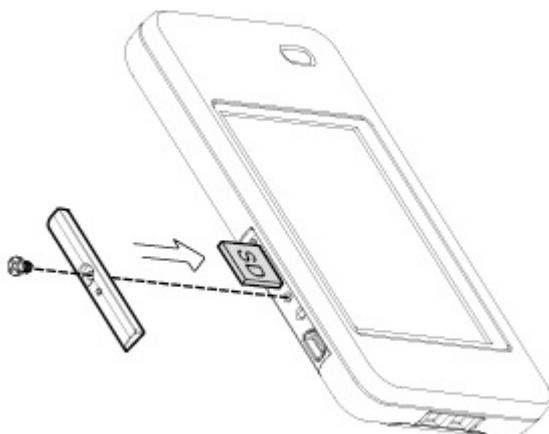
1. Release the screws (x1) to open the I/O cover on the side of the mobile system.
