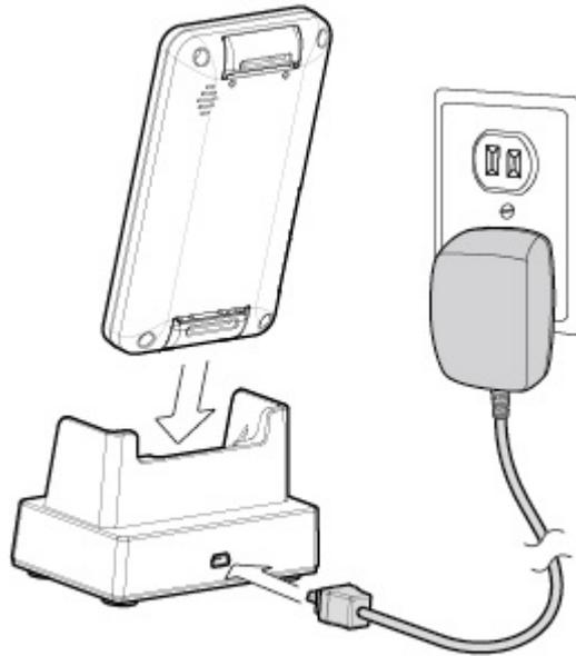
1. Connect the mini USB connector of the AC-USB adapter to the rear of the single-slot system charging cradle.
