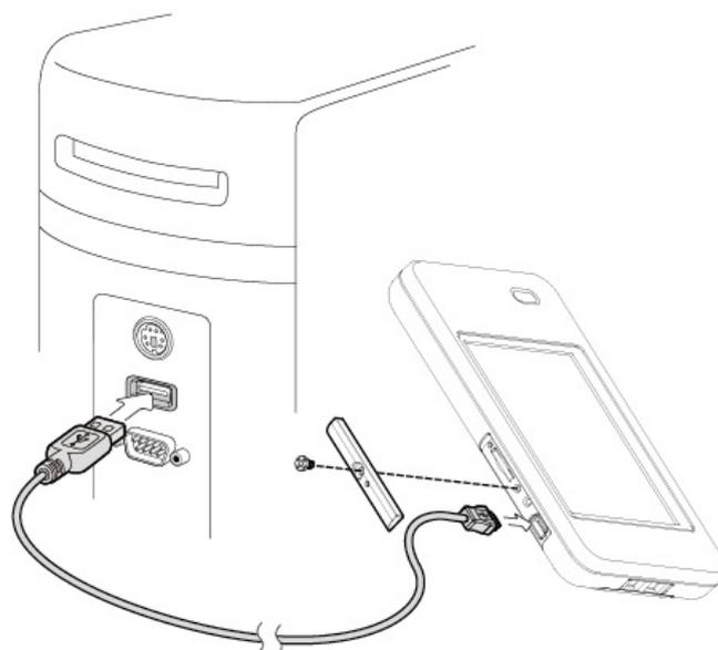
1. Unscrew the screw (x1) to open the I/O cover and connect the mini USB connector of the USB cable to the respective connector on mobile system and the USB connector to a PC.
