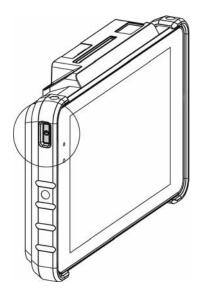
1. Push the power button to turn on the system and hold  $4\sim5$  seconds to turn off the system.
