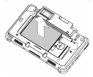
To remove the battery pull the plast ic tab aside and gently lift the battery out of the system.
