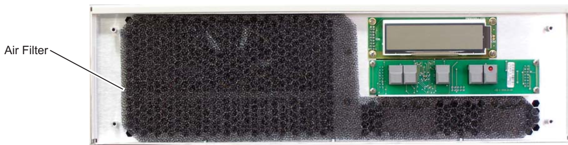
Figure 2-6. Remove the Exposed Air Filter
