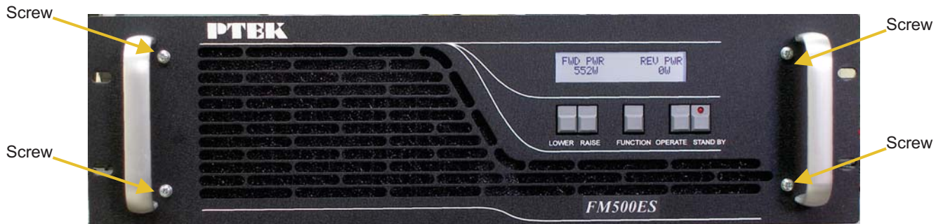
Figure 2-5. Remove the Front Panel Screws to Access the Air Filter
