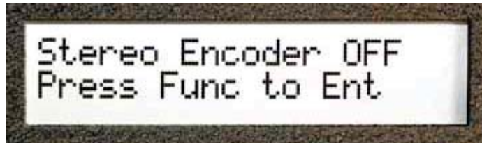
Figure 3-5. Stereo Encoder Can be Changed Through the LCD Display
