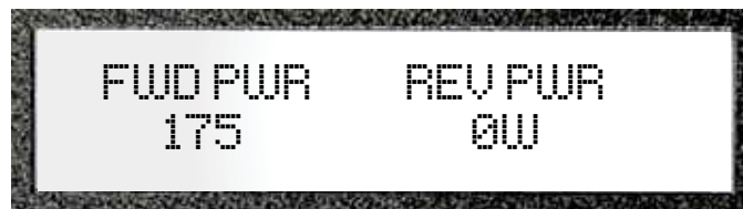
Figure 3-12. Press the FUNCTION Key to read Forward & Reverse Power
