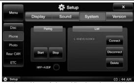
⑥ If a unique address of the mobile phone is created in the list (authentication list) on the right, the authentication process is normally terminated.
