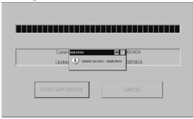
⑤ If the update is successfully completed, the screen will return to ①. Please check the updated version. If the update is completed, the main menu will appear; if the MICOM update is completed, the unit power will be automatically turned Off and On.
