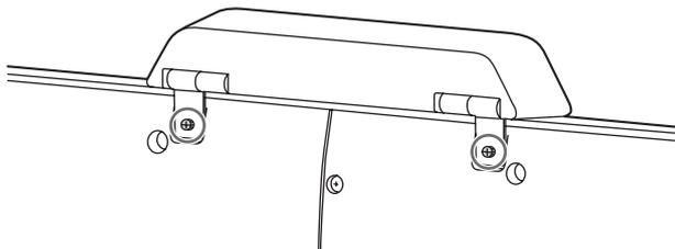
1. Attach the supplied camera with the supplied knurled screws (M3) (x2).
