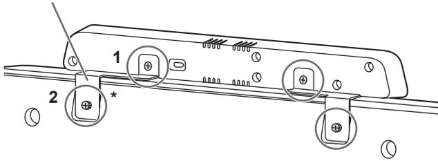
1. Attach the supplied IoT sensor hub mounting brackets (L/R) to the IoT sensor hub with the supplied IoT sensor hub screws (M3) (x2).
