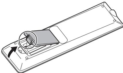
2. See the instructions in the compartment and put in the batteries (supplied with the PN-ZR02 (optional)) with their plus (+) and minus (-) sides oriented correctly.
