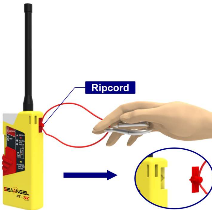
Figure 11: Activating the emergency alarm using the ripcord
