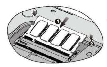
Putting the RAM model into the slot, just like the chart 20° obliquity. Pressing the two ends of card hook locked.
