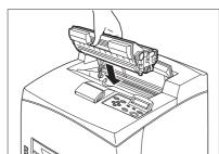
4 Hold the EP cartridge by the grip and insert it into the slot inside the printer.
