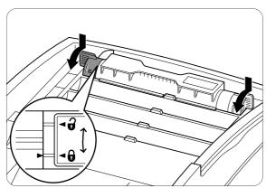
Grip the levers at each end of the toner cartridge with your fingers, then push down firmly to rotate the levers forward.
