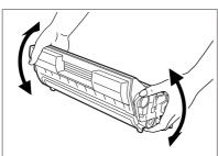
Take the EP cartridge out of the box and shake it 7 to 8 times as shown in the diagram.
