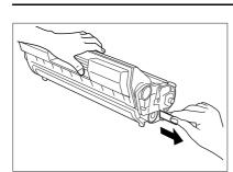
Place the EP cartridge on a flat surface and pull the seal out horizontally.
