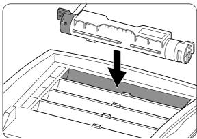
Align the toner cartridge with the corresponding insertion point in the printer and insert it as shown in the illustration.
