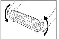
Take the EP cartridge out of the box and shake it 7 to 8 times as shown in the diagram.
